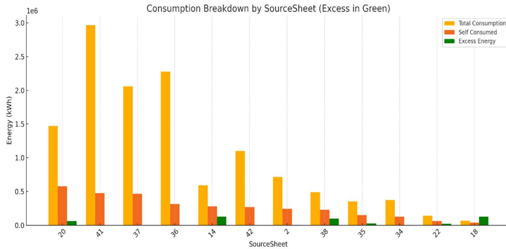
Figure 5.8: Total consumption, production, and self-consumed energy for buildings inside cabin 05.
