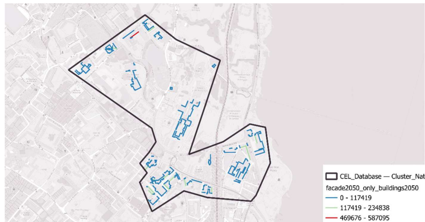
Figure 7.8: Façade production kWh/y
